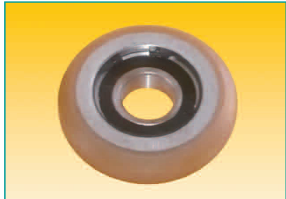
Roller VSL Ø 100/30 x 25 mm, VU-coating 80° Shore A, conical, steelring, ball bearing 6206 2RS, Art.no. 452 009
